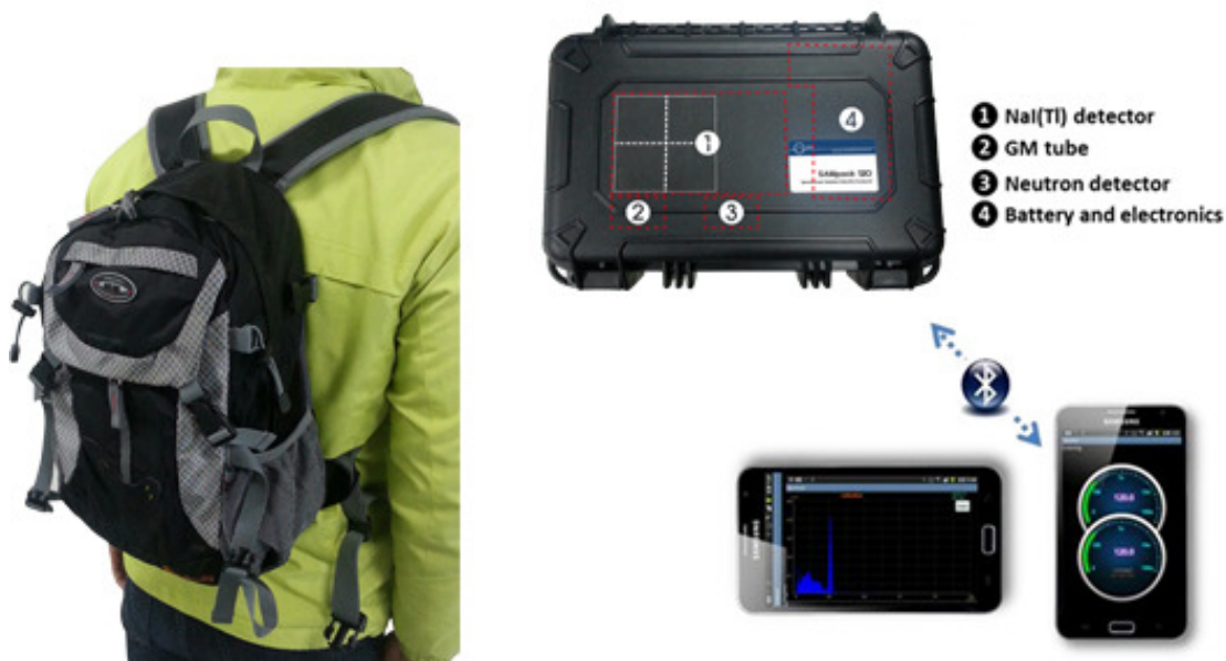
Figure 1.1. SAMpack120 Spectroscopic Radiation Detection Backpack (including optional GM tube and neutron detector)
