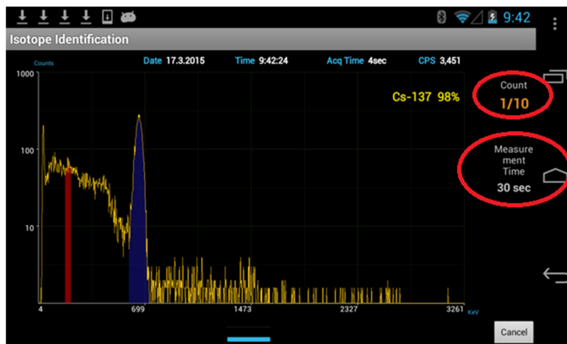
Figure 4.28. Sequential mode event capture example
