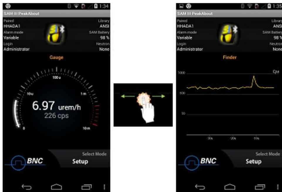
Figure 4.31. Gauge mode and Finder mode example
