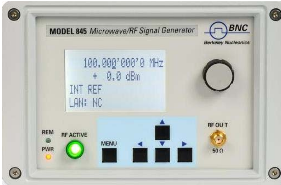
Figure 1-a BENCHTOP MICROWAVE SOURCE Front Panel View (Model MODEL 845)
