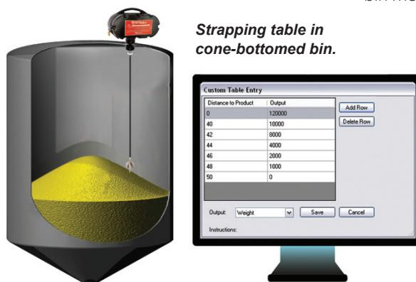
of the cone. Strapping table data also allows for more accuracy in measuring irregular tanks, such as a cylindrical tank installed on its side.
