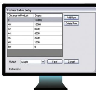
of the cone. Strapping table data also allows for more accuracy in measuring irregular tanks, such as a cylindrical tank installed on its side.
