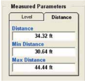
The main display screen shows average distance, as well as minimum and maximum distances.
