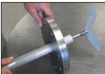
The collapsible paddle "squeezes" shut to insert into the bin and then automatically "pops" open.
