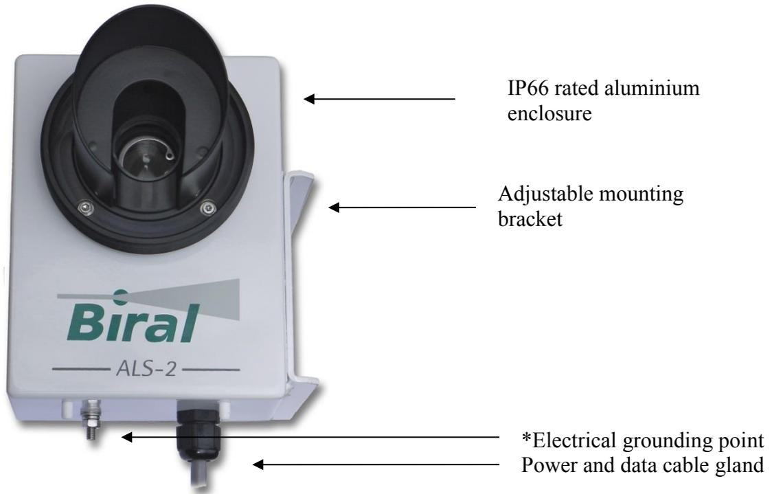
Figure 1: Main components of the Biral ALS-2
