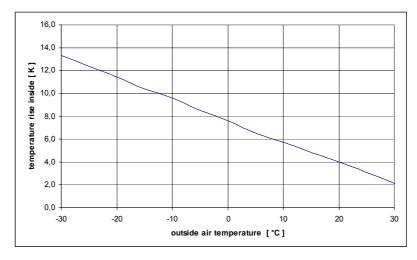
Outside - inside - difference temperature by using the heating.
