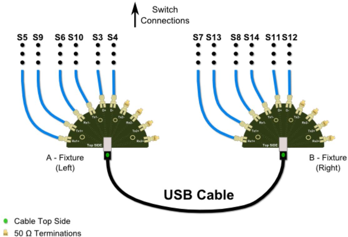
Figure 51: Connection diagram for First SS Pair measurements with Switch System
