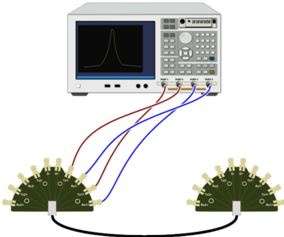
Figure 31: Connection diagram for First SS Pair measurements – A\_TX1 - A\_RX1 Pair
