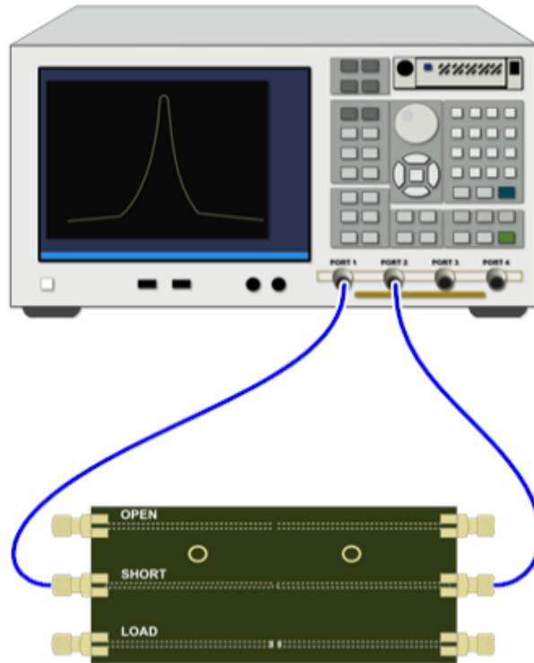
Figure 13: Connection diagram for TDR Calibration – Short 1:2
