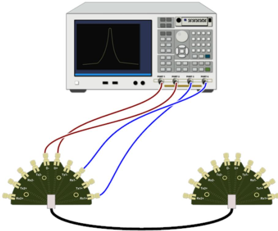
Figure 37: Connection diagram for First SS Pair measurements – A\_D - A\_RX1 Pair
