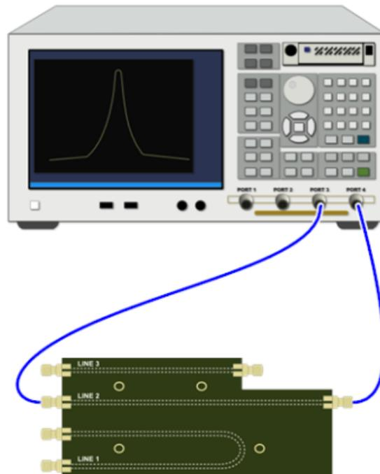
**Figure 20: Connection diagram for TDR Calibration - Line 2 Ports (3-4)**
