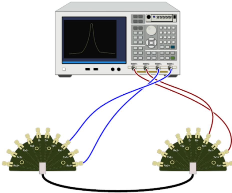
Figure 30: Connection diagram for First SS Pair measurements – B\_TX1 - A\_RX1 Pair
