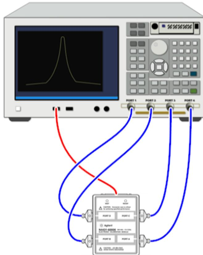
Figure 10: Connection diagram for ENA Initial Configuration
