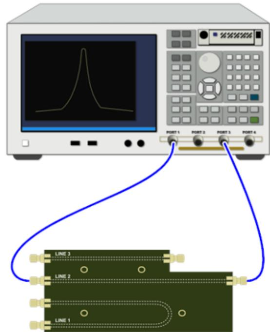
**Figure 19: Connection diagram for TDR Calibration - Line 2 Ports (1-3)**
