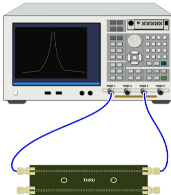
**Figure 12: Connection diagram for TDR Calibration – Thru 1-3**
