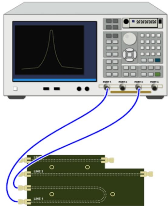
**Figure 16: Connection diagram for TDR Calibration -
