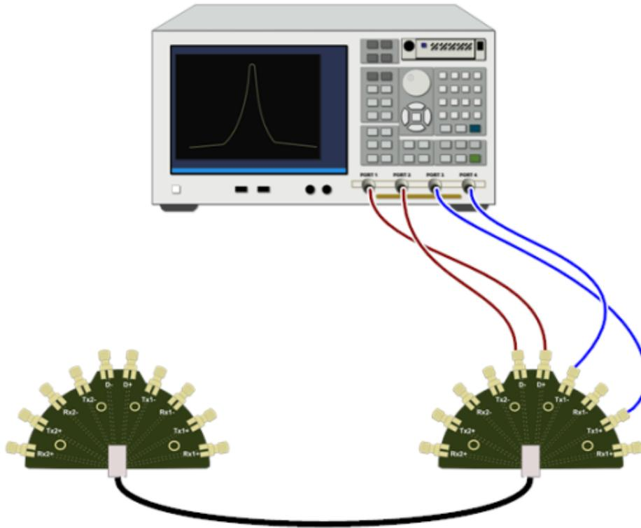
Figure 40: Connection diagram for First SS Pair measurements – B\_D - B\_TX1 Pair
