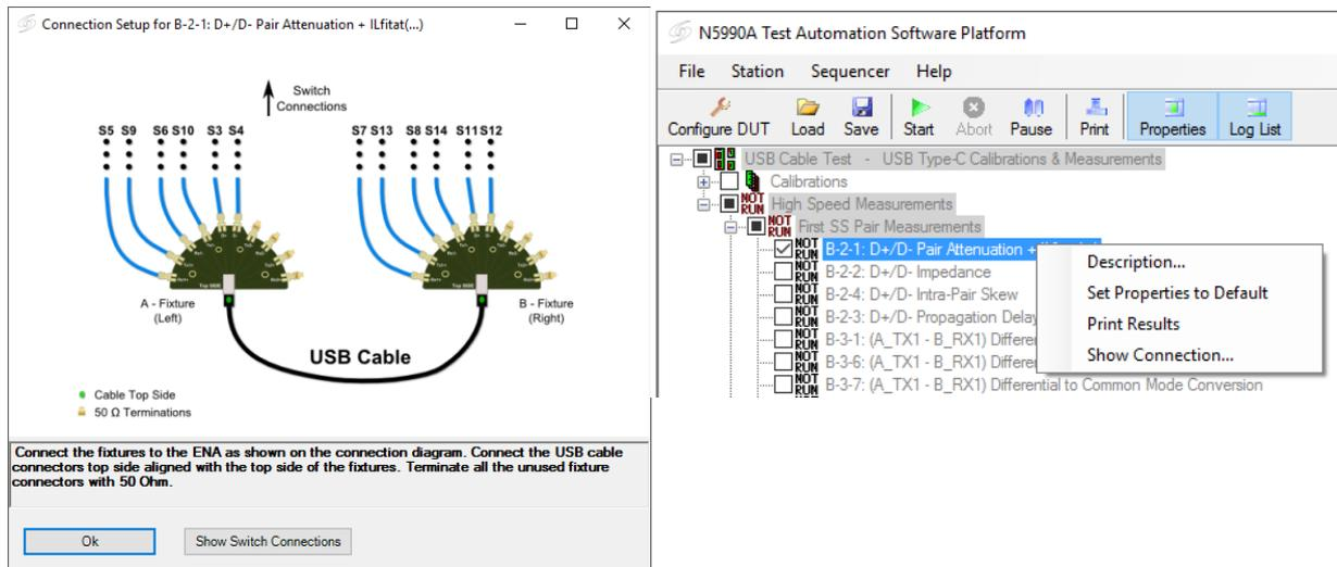
**Figure 9: Showing Connection Diagram dialog**
