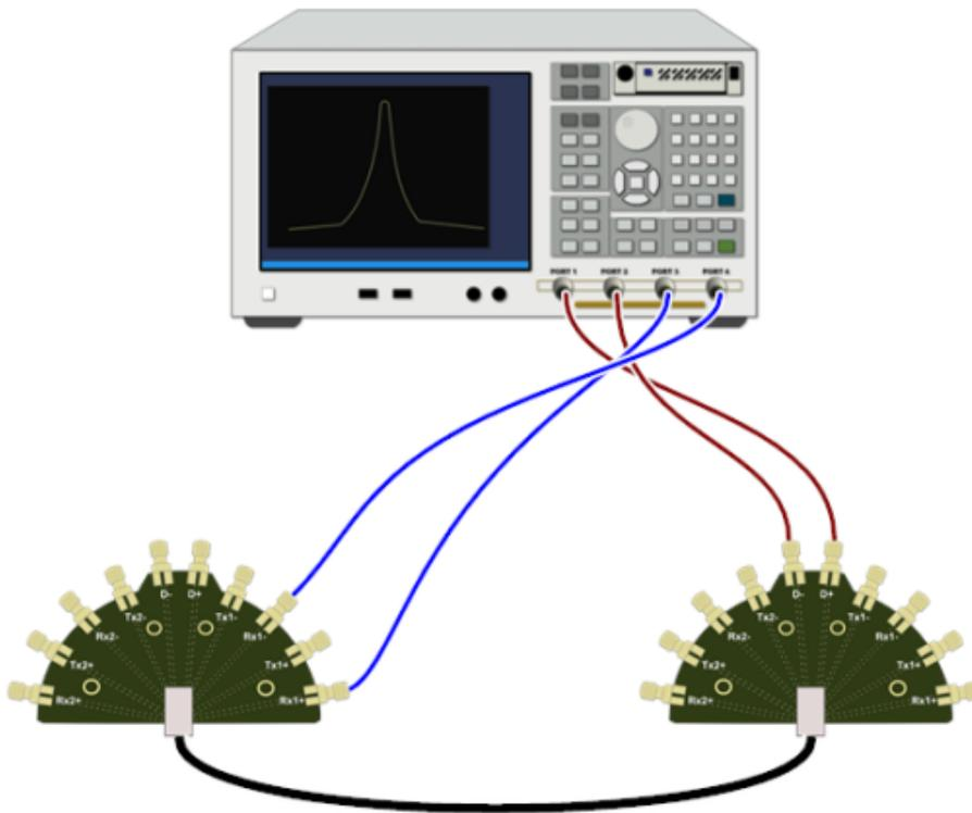
Figure 43: Connection diagram for First SS Pair measurements – B\_D - A\_RX1 Pair
