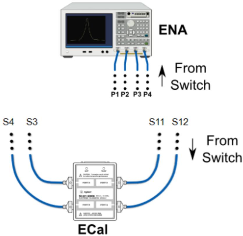
Figure 49: Connection diagram for Switch Ecal Calibration
