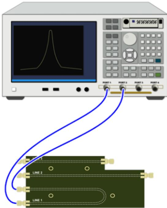
**Figure 15: Connection diagram for TDR Calibration -
