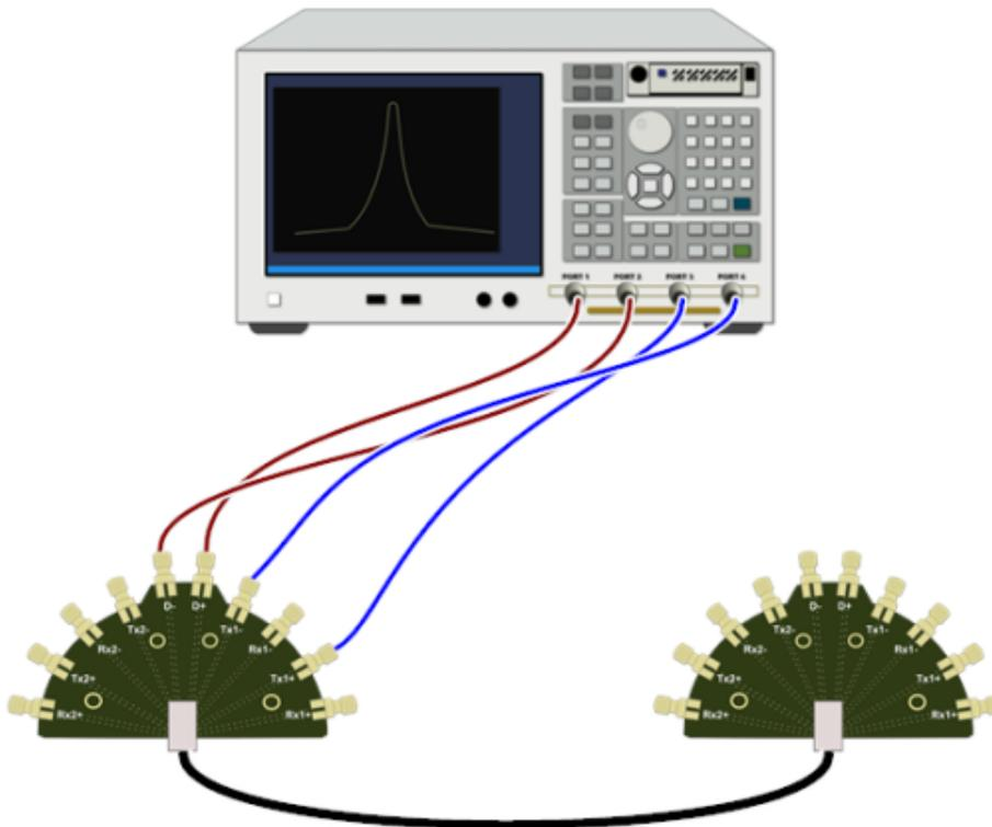
Figure 36: Connection diagram for First SS Pair measurements – A\_D - A\_TX1 Pair
