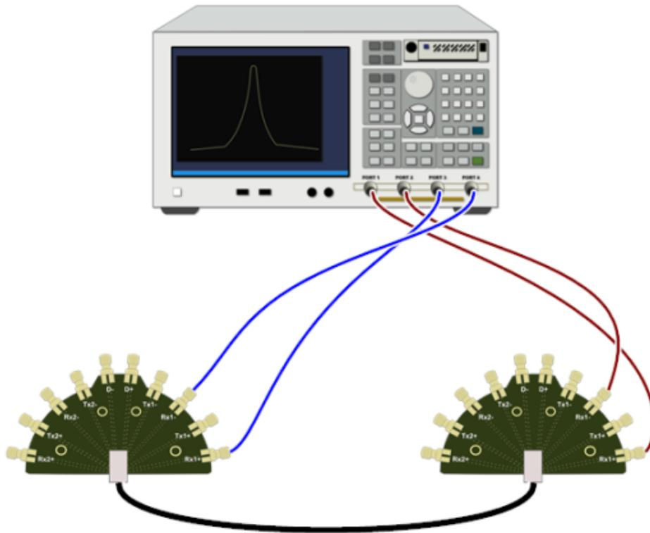
**Figure 34: Connection diagram for First SS Pair measurements – B\_RX1 - A\_RX1 Pair**
