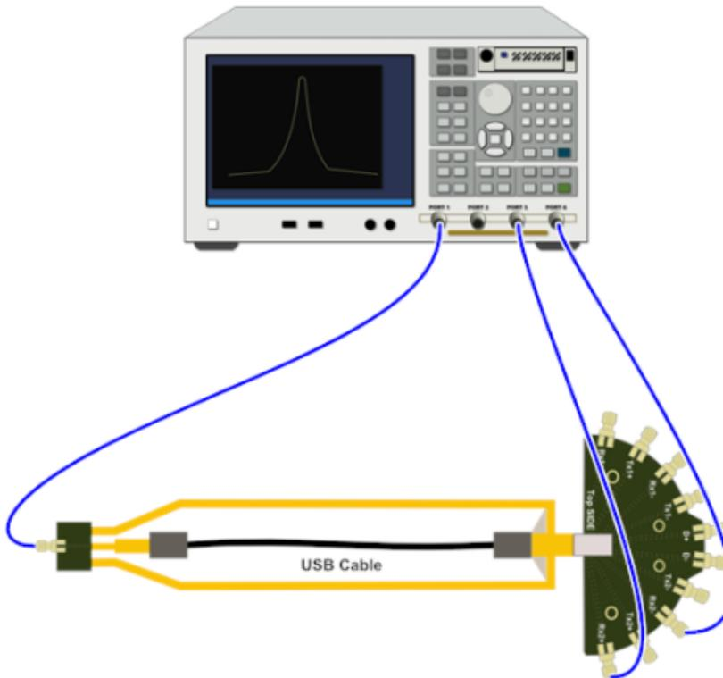
Figure 47: Connection diagram for Shielding Effectiveness - B\_RX2
