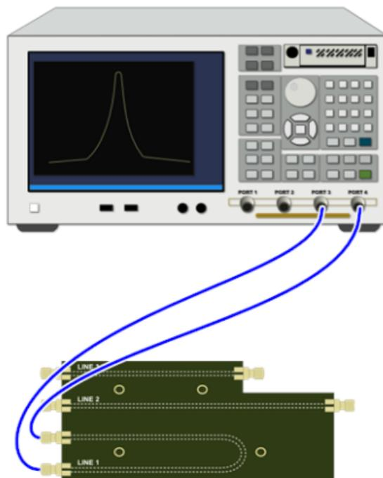
**Figure 17: Connection diagram for TDR Calibration –
