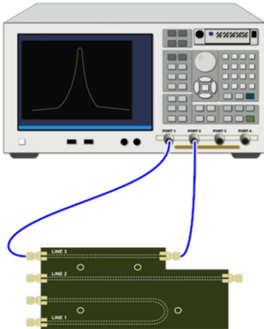
**Figure 21: Connection diagram for TDR Calibration -
