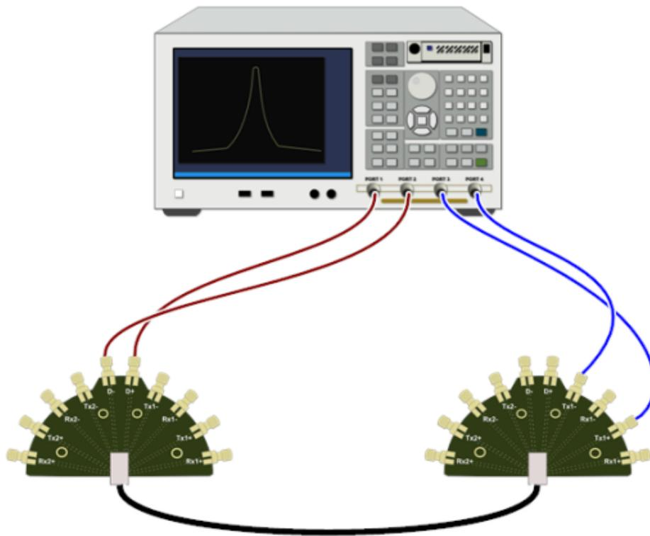
Figure 38: Connection diagram for First SS Pair measurements – A\_D - B\_TX1 Pair
