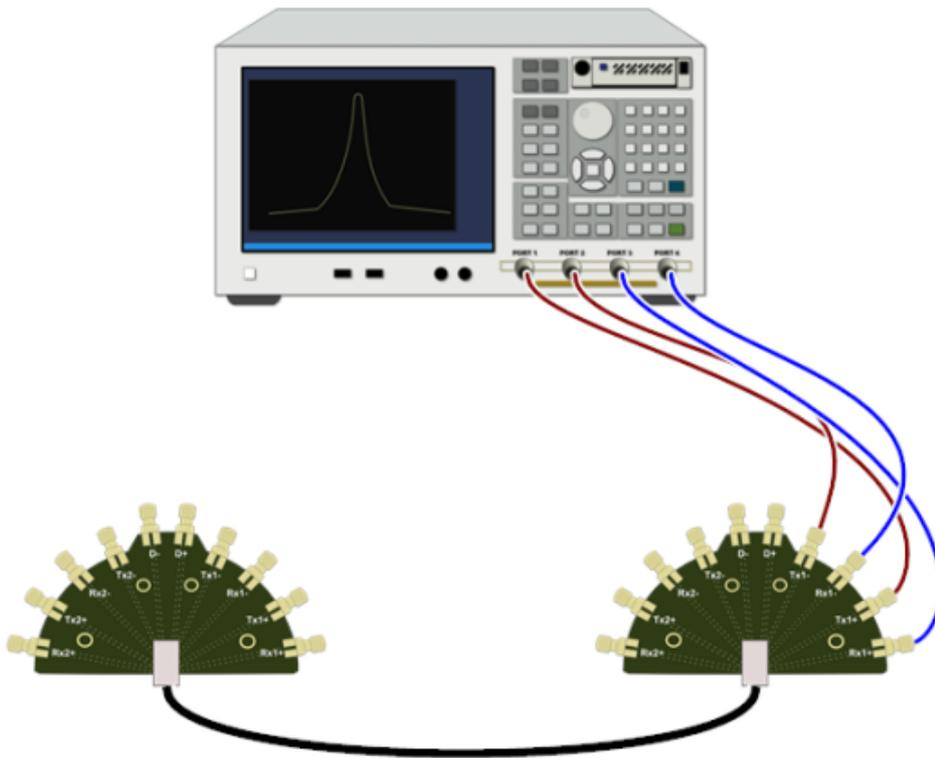
Figure 32: Connection diagram for First SS Pair measurements – B\_TX1 - B\_RX1 Pair
