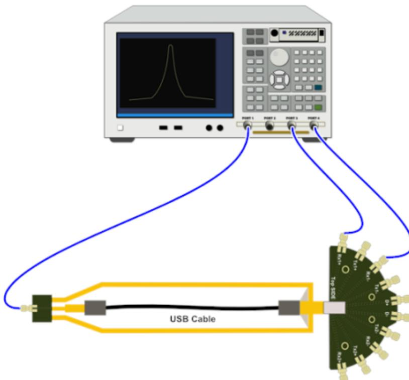
Figure 45: Connection diagram for Shielding Effectiveness - B\_RX1
