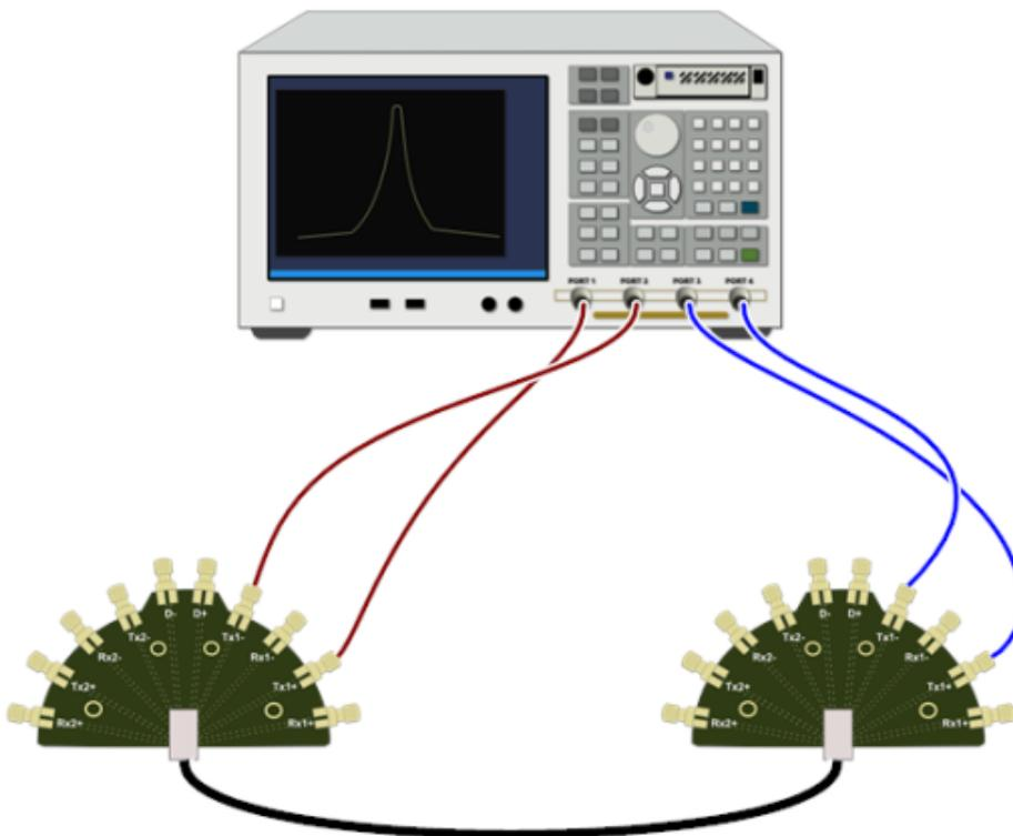
Figure 33: Connection diagram for First SS Pair measurements – A\_TX1 - B\_TX1 Pair
