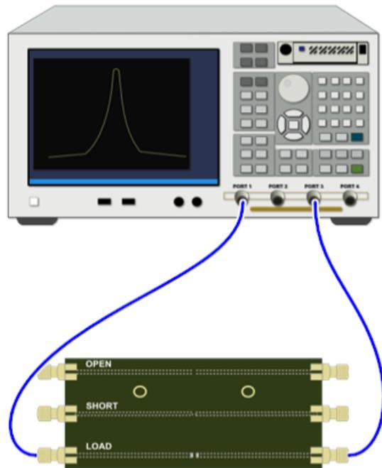
**Figure 25: Connection diagram for TDR Calibration - Load Ports (1-3)**
