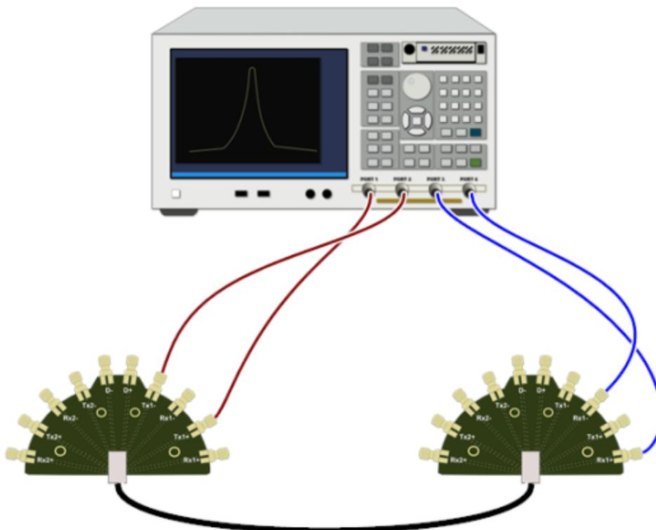
Figure 29: Connection diagram for First SS Pair measurements – A\_TX1 - B\_RX1 Pair
