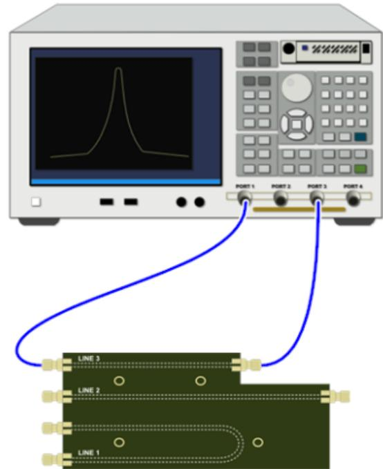
**Figure 22: Connection diagram for TDR Calibration -
