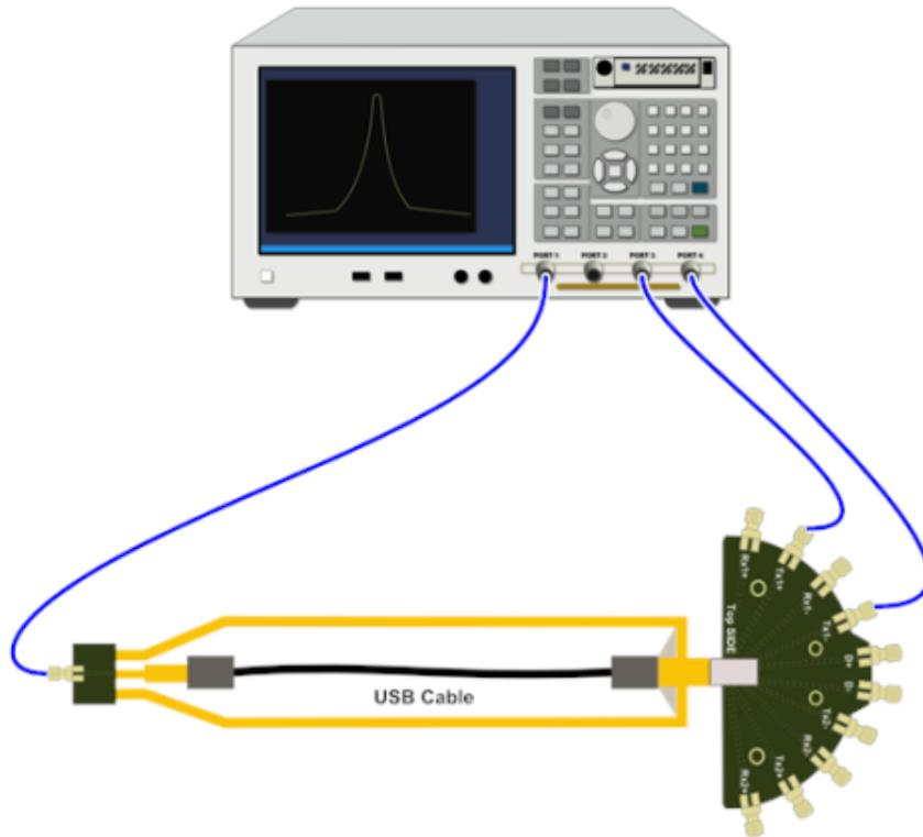
Figure 44: Connection diagram for Shielding Effectiveness - B\_TX1
