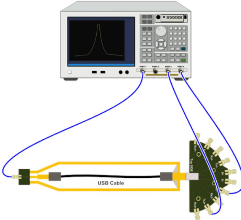
Figure 46: Connection diagram for Shielding Effectiveness - B\_TX2
