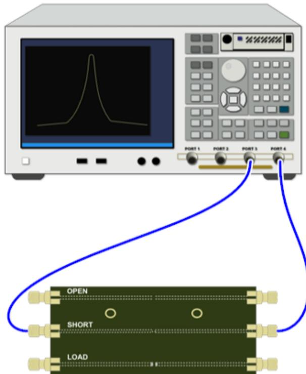
Figure 14: Connection diagram for TDR Calibration – Short 3:4
