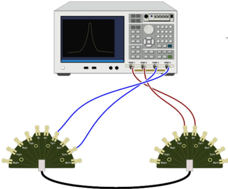
Figure 42: Connection diagram for First SS Pair measurements – B\_D - A\_TX1 Pair
