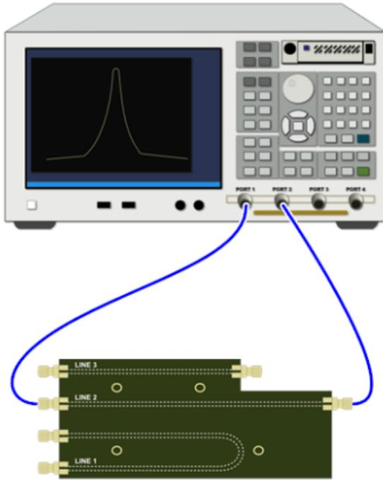
**Figure 18: Connection diagram for TDR Calibration - Line 2 Ports(1-2)**
