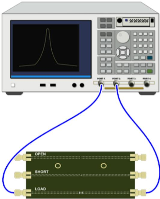
**Figure 24: Connection diagram for TDR Calibration - Load Ports(1-2)**
