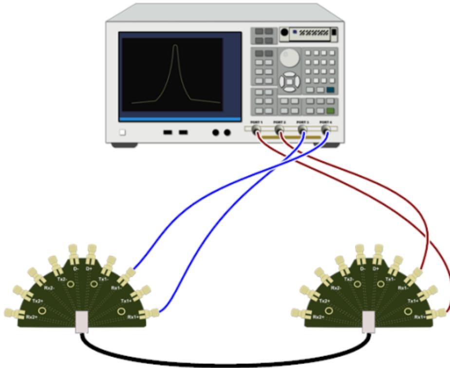
Figure 35: Connection diagram for First SS Pair measurements – B\_RX1 - A\_RX1 Pair
