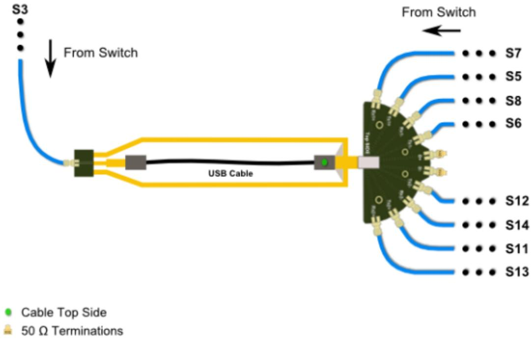
Figure 52: Connection diagram for Shielding Effectiveness measurements with Switch System
