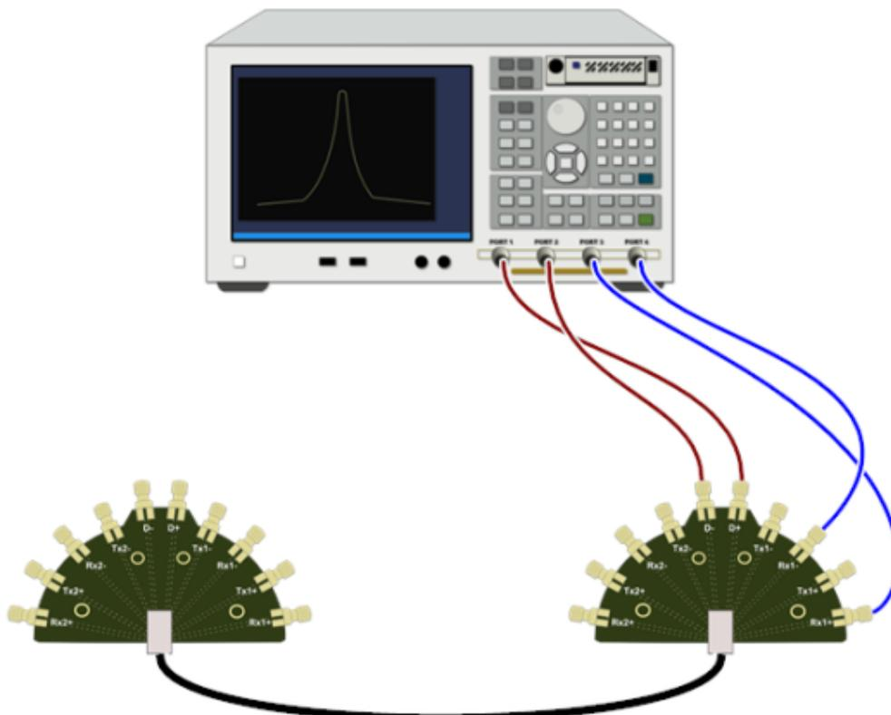
Figure 41: Connection diagram for First SS Pair measurements – B\_D - B\_RX1 Pair
