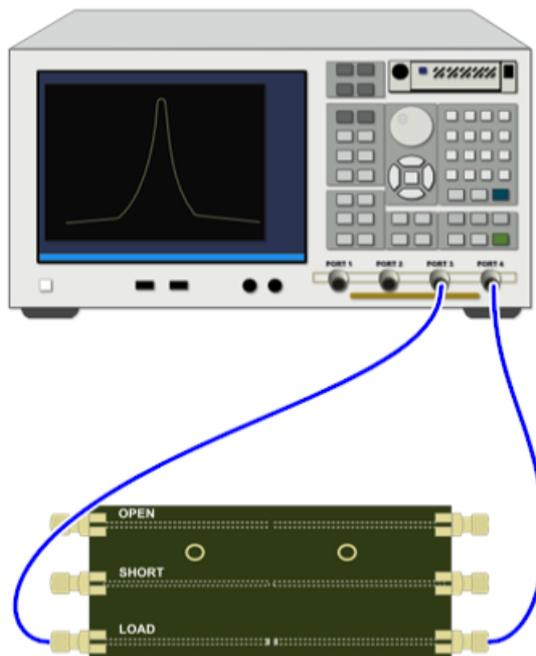
**Figure 26: Connection diagram for TDR Calibration - Load Ports (3-4)**
