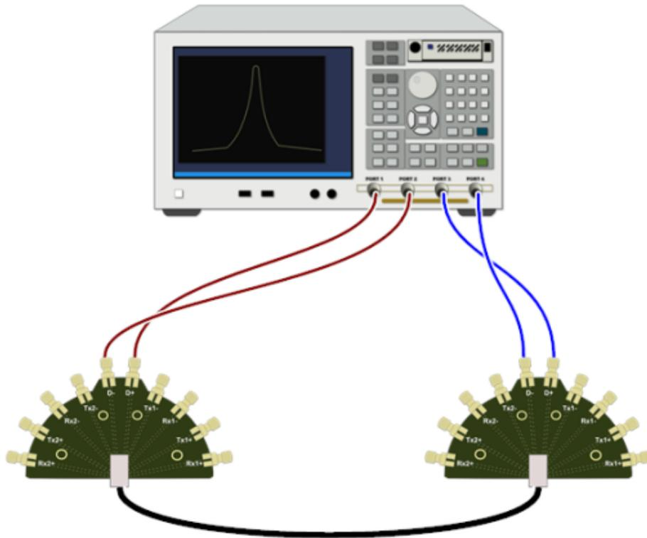
Figure 28: Connection diagram for First SS Pair measurements – D+/D- Pair
