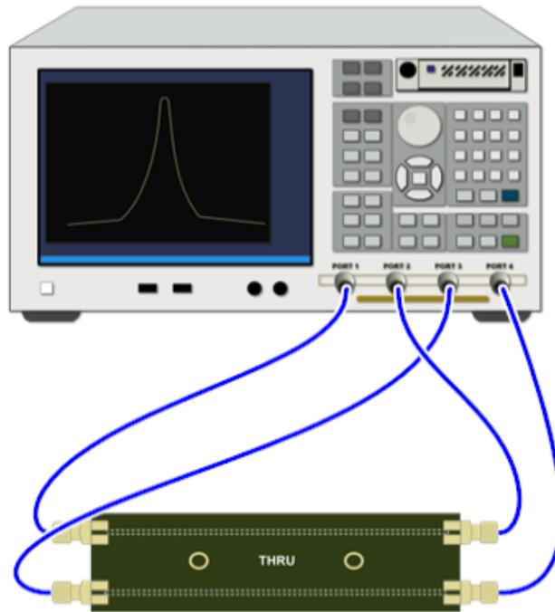
**Figure 11: Connection diagram for TDR Calibration – Thru 1-2:3-4**
