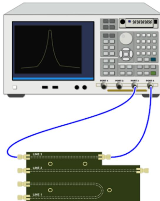
**Figure 23: Connection diagram for TDR Calibration –
