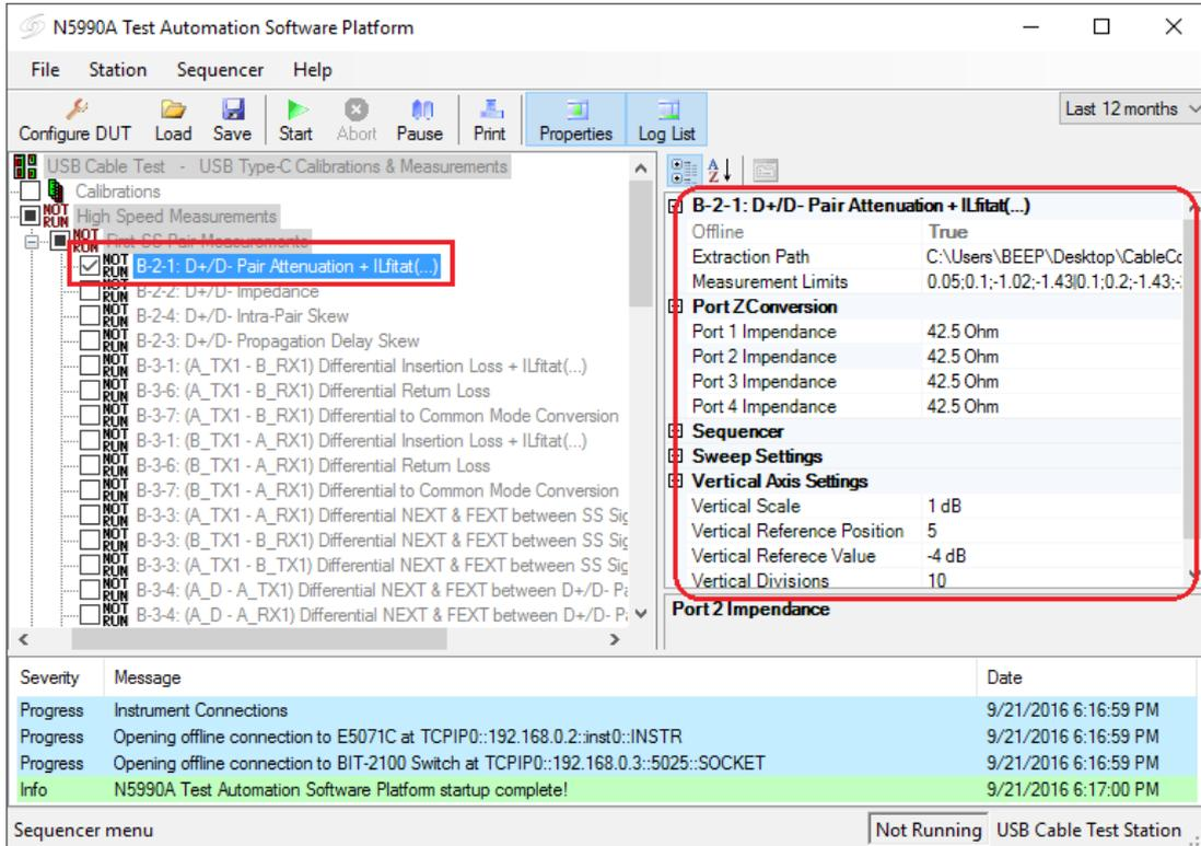
Figure 8: Modifying Procedure Parameters
