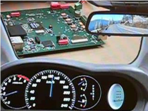
BADGE works as a graphics engine in embedded systems, but doesn't suffer from the short life cycles affecting the usual graphics controllers. It is very flexible. Can interface to numerous types of processors, memories and displays.
