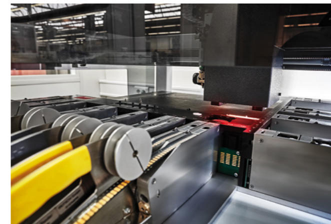
LED assembly is carried out in our own ESD-protected facilities.
