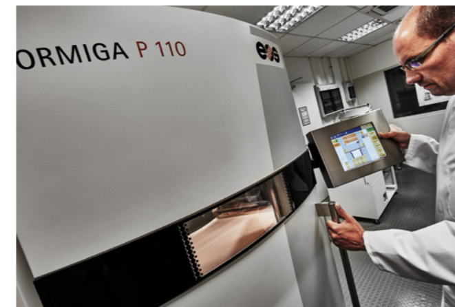
Plastic laser-sintering systems enable fast, economical production of small batches and individual solutions, even with geometrically complex designs
