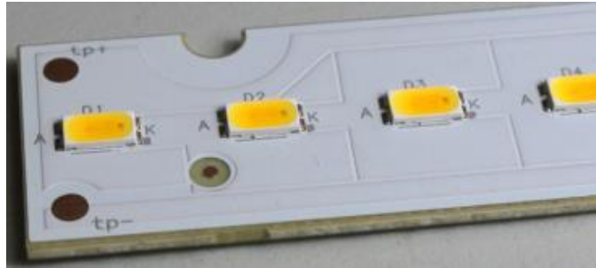
Example - 20 mm-wide LED module with open fixing hole
