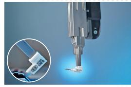
Electronic control gear can also be parameterised by the insertion of a resistor on the secondary side. To make this method as easy as possible, we have developed the Set'n'Drive resistor, which can be inserted either manually or automatically. In the case of automatic processing with an ADS wiring system, the three gripping positions enable the wiring tool to insert resistors at
