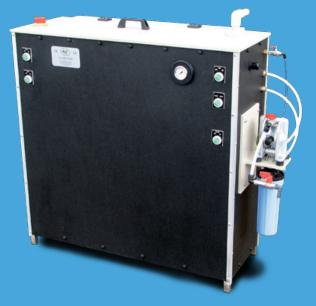
The stencil is immersed in the agitated solution for 5-10 minutes then either removed and left to dry in the holder on top of the machine (see photo on right) or slowly withdrawn passed the twin air knives (VSCM/D model only, see photo on right)
