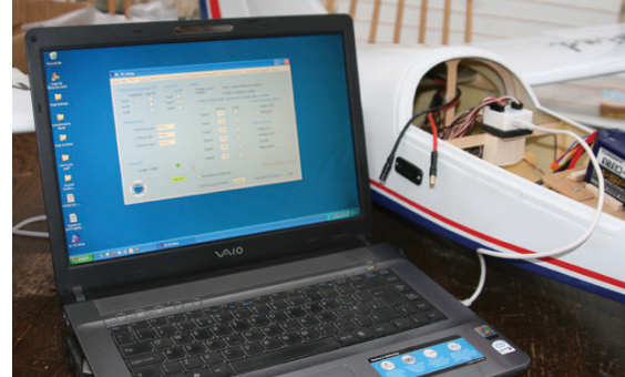
Setting up the BL-3G in the Seawind. Gyro is upright and sat on a foam mat.
