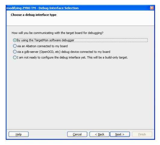
Enter your ZYBO's IP address in the next panel, getting the address from the terminal window that shows the bootrom application's start-up. The IP address is on the last line. Leave the port number as 2001.
