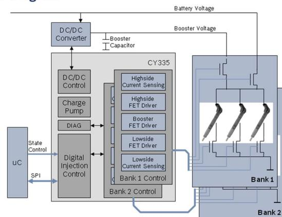
CY335 contains a digital control part, a driver for the DC/DC converter and two identical output stage banks, each of which can drive up to three injectors. Optionally, bank 1 can control up to four injections if bank 2 is not used.
