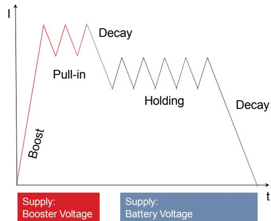
During opening phase of the injector, the current is supplied from the booster voltage. To keep the injector open, the CY335 switches from the booster FET to the highside FET and reduces the current through the injector. At the end of the injection, the current decays back to zero.
