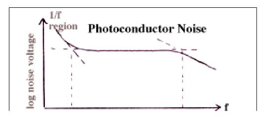
To predict low frequency performance of a photoconductor, the extent to which  $D^*$  is degraded by 1/f noise must be estimated. Either of the following ways is applicable:
