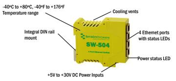
Industrial DIN mountable Ethernet Switch Devices (-40°C to +80°C, -40°F to +176°F Temperature range)
