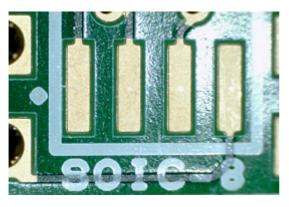
Close up to show the solder mask with protecting windows around the pads, to minimize the risk of solder bridges, when the SOIC is hand soldered.
