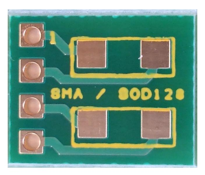
In above photo is visible the green solder mask around the pads and protecting the tracks in this adapter.
