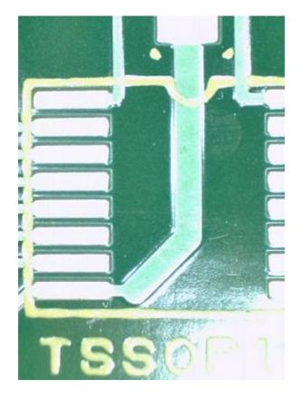
Solder mask exist only around pads and is used to minimize the risk of building solder bridges between pads, that easy to happen when the device is hand soldered.
