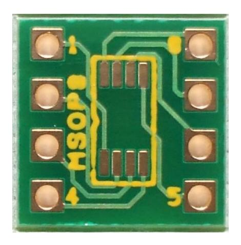
In above photo is visible the green solder mask around the pads and protecting the tracks in this adapter.
