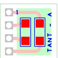
**Applications of this adapter:** small pcb board for hand soldering prototypes with up two SMD components.
