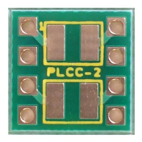
In the photo is possible to see the green solder mask around the pads and protecting the tracks in this adapter.
