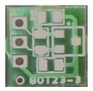
Accept row 3 pin connectors with 2,54 mm pitch, breadboard compatible. This adapter is foreseen for up to 3 decoupling capacitors of 0805 type between any legs. Available a ground connection. Ground plane works as an heatsink.
