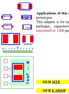
**Applications of this adapter:** small pcb board for hand soldering of SMD prototypes.
