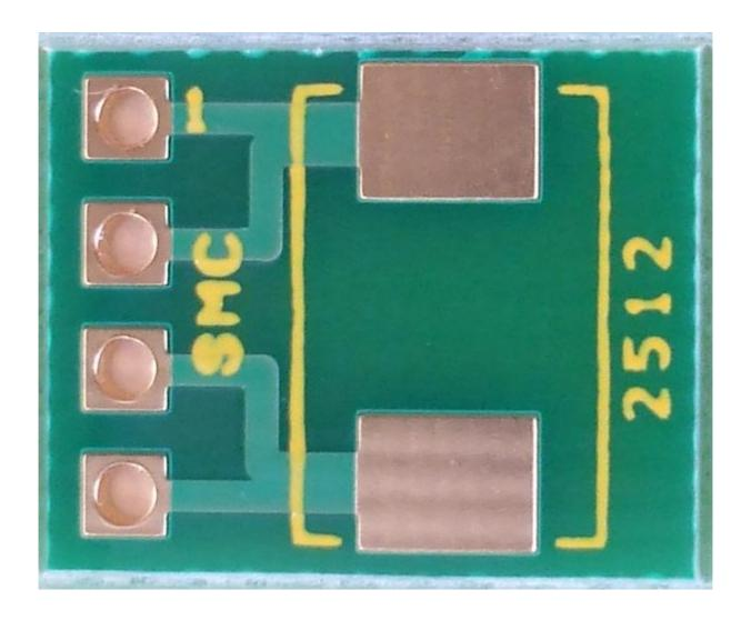
In above photo is visible the green solder mask around the pads and protecting the tracks in this adapter.
