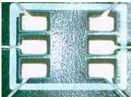
Closeup of pads to show the solder mask
