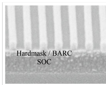
Figure 4. Multilayer system for pattern transfer showing the hardmask/BARC layer plus SOC.
