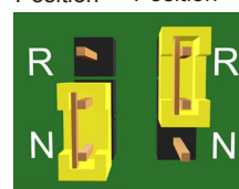
LEXP Switch Input Jumper Settings
