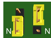
LMB Switch Input Jumper Settings
