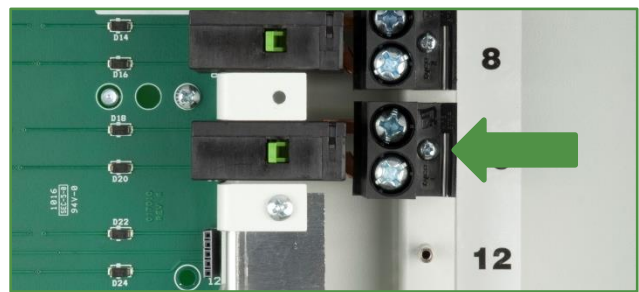
4. Secure LTR with the LTR Fastener. DO NOT exceed 5 in-lbs when tightening. 5. After inserting wire into LTR, torque each Screw Terminal to 36 in-lbs.
