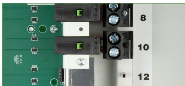
3. Install LTR by inserting the Relay Pins in the corresponding plug on the Relay Interface Board. Then gently press the LTR towards center and back of the panel until the LTR Mounting Hole seats over the mounting stud.
