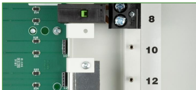
2. Remove relay blank.
