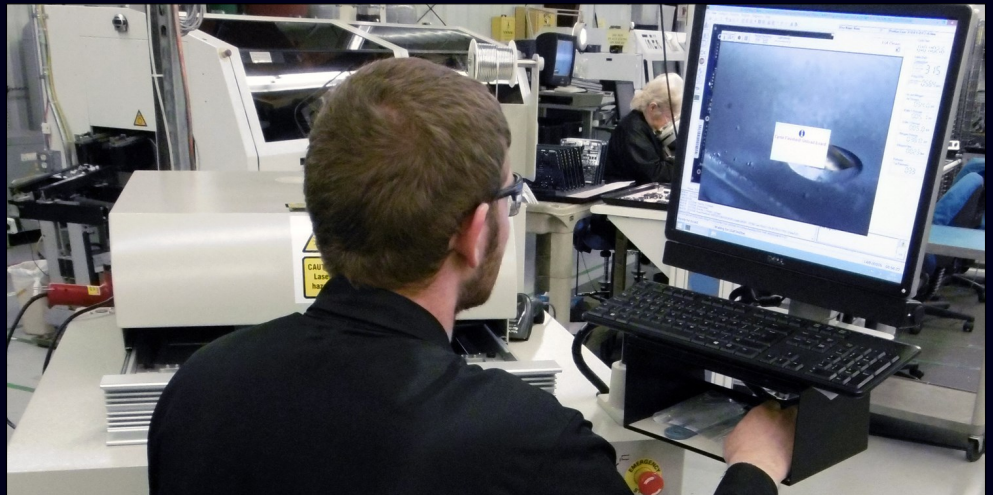
The new selective solder machines enable Burton Industries' team to run leaded and lead-free simultaneously or quickly ramp up extra capacity in either technology.
