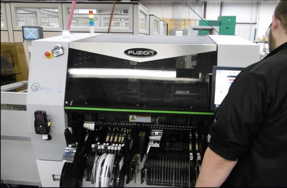
Burton Industries has added a new SMT line that includes an Advantis Fuzion F1-30 high speed placement machine and the Fuzion F1-11 flexible platform.
