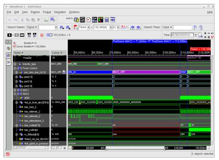
Figure 4: Engineers can determine the DUT's power characteristics very early in the project life cycle. In this example, the user is verifying a full cycle of power shut off (note the Xs in the center) and correct state restoration.
