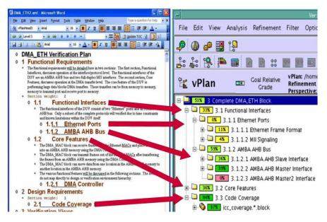
Figure 2: The Desktop Manager component of Incisive Enterprise Simulator can create an executable vPlan from a written specification. This plan is then used to drive all simulations, with the coverage results from multiple simulaton runs automatically backannotated into the vPlan for a "total coverage" view.
