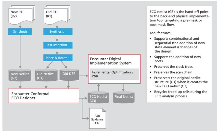
Figure 2: The Encounter Conformal ECO Designer implementation flow
