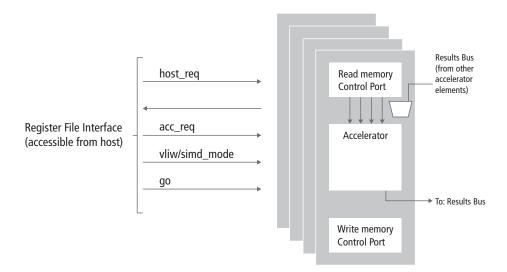
Figure 2: Base architecture for evaluation of programmable vs. hard-coded accelerators
