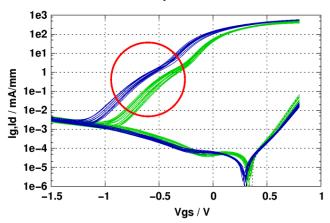
Figure1: Measurement: drain and gate leakage current for 100nm gate length transistors with two different distances between Schottky contact and channel
