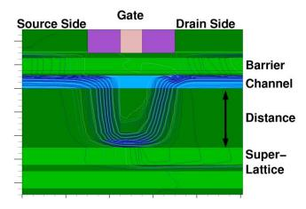
Figure 4: Device simulation: current flow lines for Lg=100nm, Vds=2.5V and Vg=-0.8V
