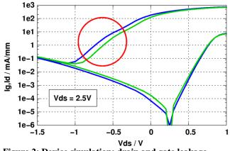
Figure 2: Device simulation: drain and gate leakage currents for 100nm gate length HEMTs with different distances between Schottky contact and channel
