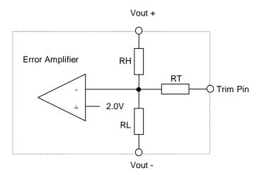
The combination of the resistors RH & RL establish an input impedance of 4.75k into the inverting input of the error amplifier (when the Trim pin is open circuit).
