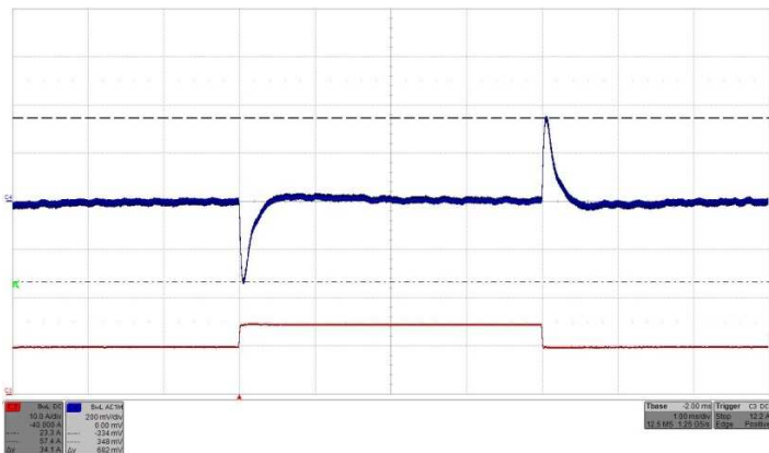
Fig. 43: Output voltage response to load current step change 50% - 75% - 50% (9.5A-14.25A-9.5A) with di/dt = 1A/\mu s at V_{in} = 24V . Top trace (C4): Output voltage (200 mV/div.). Bottom trace (C3): Load current (10A/div.). Time: 1ms/div.
