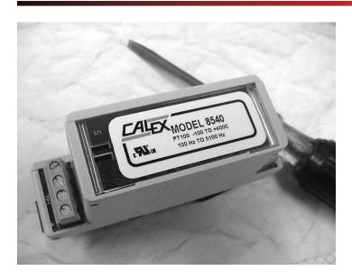
Model 8540 RTD to frequency converter is designed to operate into a common 24 volt, 7mA PLC high speed counter input. It's output is an isolated optocoupler transistor and provides DC isolation from the input and DC power. The 8540 will operate with a DC supply of 15 VDC to 26 VDC at 37 mA.
