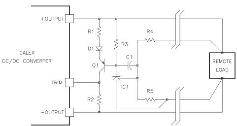
Figure 1. Remote Sense Circuit.
