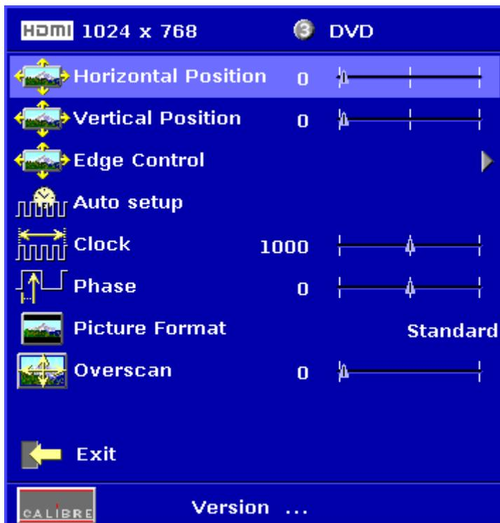
Horizontal and vertical position controls shift the image left/ right, up/ down. For graphic modes also the edges can be shifted individually within available limits. The image is scaled accordingly.
