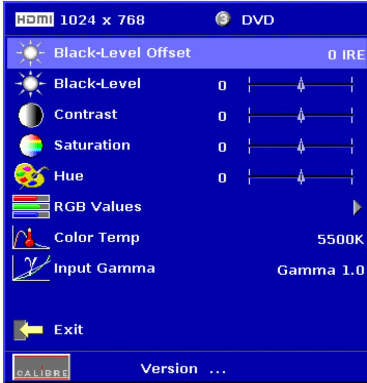
The gain and black level of each RGB channel can be adjusted individually through the RGB values menu.
