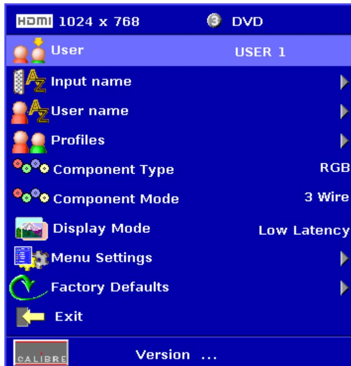
The “Display Mode” can be set to either “Low Latency” mode or “Best Picture” mode. In “Best Picture” mode optimum image processing is applied, whereas in “Low Latency” mode the lowest latency is achieved. The flicker of interlaced video is not suppressed totally for the latter setting. Thus it has the disadvantage of conventional CRT TVs, but also their advantage of almost no delay in response, which is important for applications such as gaming, simulation or imaging in medical treatment.
