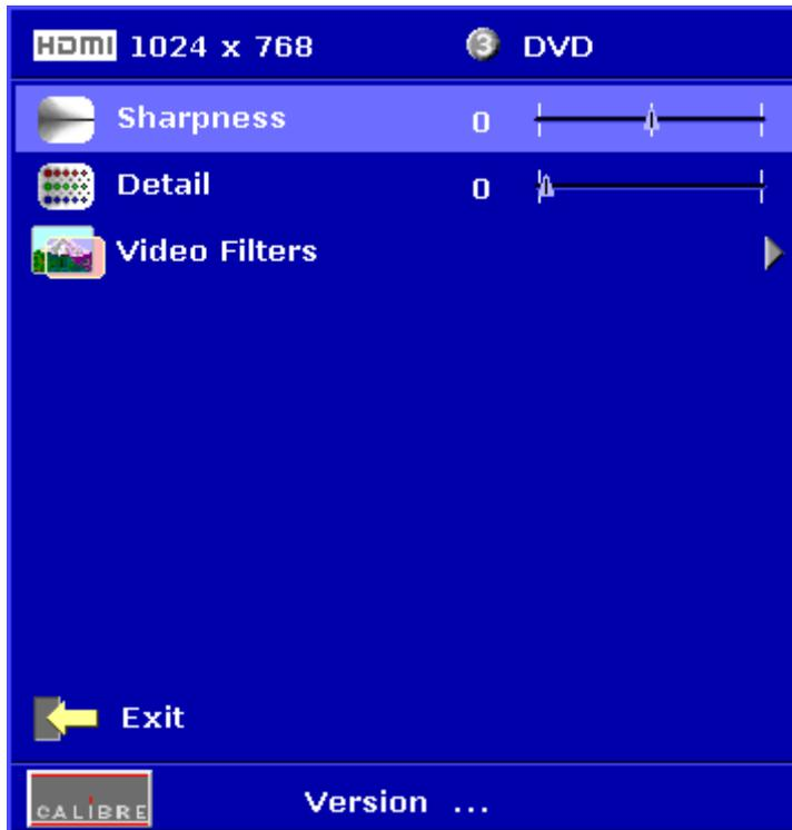
The video filters menu allows to change the level of various filters. The LTI filter enhances the sharpness of the luminance component. The CTI filter enhances the color sharpness of the chrominance signal by increasing the steepness of color edges.
