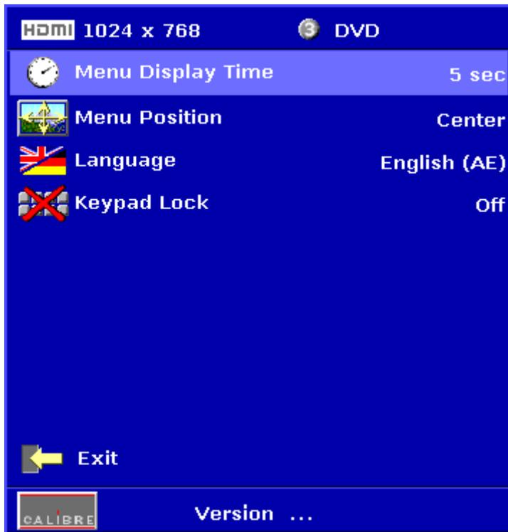
The menu language can be altered and the keypad can be locked. To unlock the keypad a combination of keys has to be pressed at the same time. This is by pressing Menu, Br- and Br+ for the standard keyboard.
