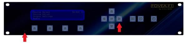
Press and hold the Right arrow key and then press the recessed reset key. The unit indicates it is Ready for update with a message in the front window.
