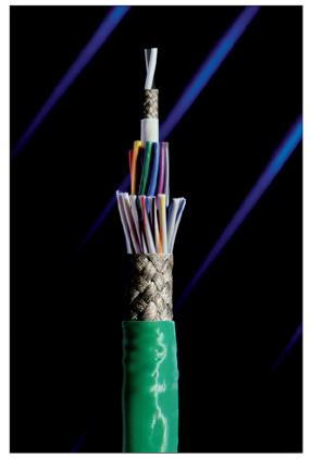
Figure 1. A cable with two Aracon shields. The inner shield, over a four-conductor group, keeps EMI from the control wires from interfering with the sensor signals.
