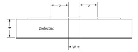
One of the advantages of a coplanar waveguide is the ability to change the width of the microstrip whilst maintaining the characteristic impedance of the transmission line.
