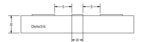
• A variant of coplanar waveguide is formed when a ground plane is provided on the opposite side of the dielectric, which is called *finite ground-plane coplanar* waveguide.
