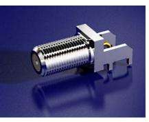
applications. With an impedance of 75 ohm and a reflection factor (VSWR) of 1.3 Max between 0.0 and 3.2 GHz this F connector is uniquely positioned for use in high speed broadcast satellite communication systems.
