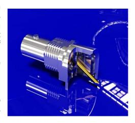
DIN 1.0/2.3 options include a Top Entry Bulkhead PCB mounting type and also a two part Top Entry version where the "inner" is PCB mounted and the "outer" detaches to facilitate board swapping without the necessity of removing attached patch cables.
