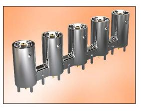
contributes to reduced handling and assembly costs in production. With a Reflection Factor (VSWR) of 1.28 between DC and 6.0GHz and an impedance of 75 Ohms this coaxial connector array is designed specifically for use in 3G-SDI broadcast applications.
