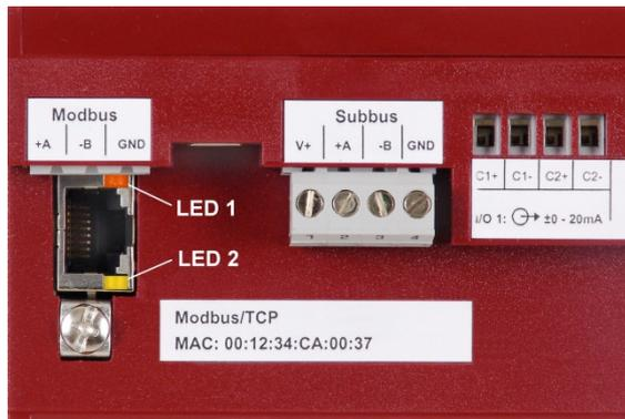
The standard RJ45 connector serves for direct connecting an Ethernet cable. If the PC is directly connected to the device a cross-wired cable must be used.
