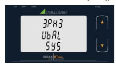
Pressing the " Down" key will enter into the "System Type edit" mode. For Active / Apparent / Reactive Power Transducer, System type will scroll between
