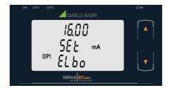
Confirmation of Elbow value Pressing the " Down" key will re-enter into the "Elbow value edit" mode.
