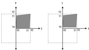
X0 = Start value of input Y0 = Start value of output X1 = Elbow value of input Y1 = Elbow value of output Y2 = End value of input Y2 = End value of output
