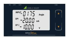
For Phase Angle Transducer Input Phase Angle Output 1 as Current or Voltage and Output 2 as Current or Voltage
