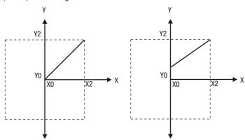
2) Example of setting with Bent characteristics:
