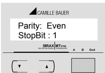
Pressing “DOWN” key re-enters into the Parity and stop bit Edit menu.
