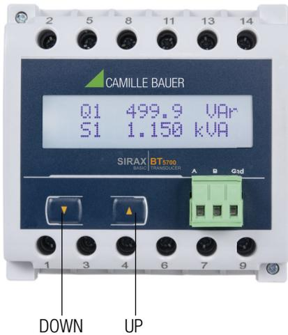
SIRAX BT5700 can be configured and programmed at site for the following: PT Primary, CT Primary, CT Secondary (5A or 1A) & three wire, three phase system or four wire, three phase system. The front panel has two push buttons through which the User may scroll through the available measurement readings, reset the energy (Import/Export) Min/Max (System Voltage & System Current) & configure the product.
